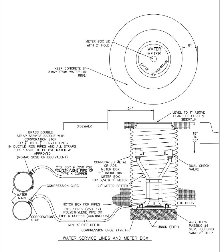
NOTE: 1.5" AND LARGER WATER METER SHALL CONFORM TO STANDRAD FOR LARGE METERS. SEE DRAWING #LCM-1
