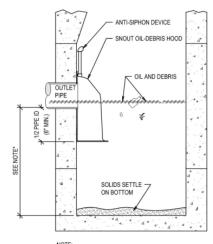
$\frac{\text{NOTE:}}{\text{SUMP DEPTH OF 36"}} \frac{\text{MIN.}}{\text{FOR}} + \text{OR} = 12" \text{DIA.} \text{ OUTLET.}$  FOR OUTLETS > OR= 15", DEPTH = 2.5 TO 3 X's DIAM.
