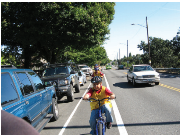
Bike lanes are delineated from the adjacent travel lane by a painted line parallel to the lane
