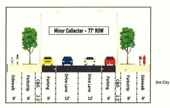
Developer agree to an alternative road cross-section in the future, all interior roads in the Project shall be constructed according to the following 53-foot wide local road section (EMMC table 16.35.130(b)):
