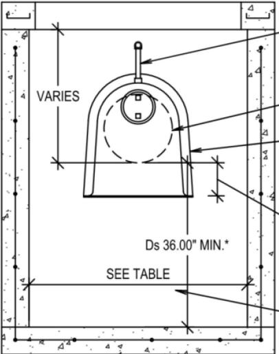
ANTI-SIPHON VENT STACK SIZED ACCORDING TO TOP OF STRUCTURE OR GRATE. 3" MIN. HEIGHT.
