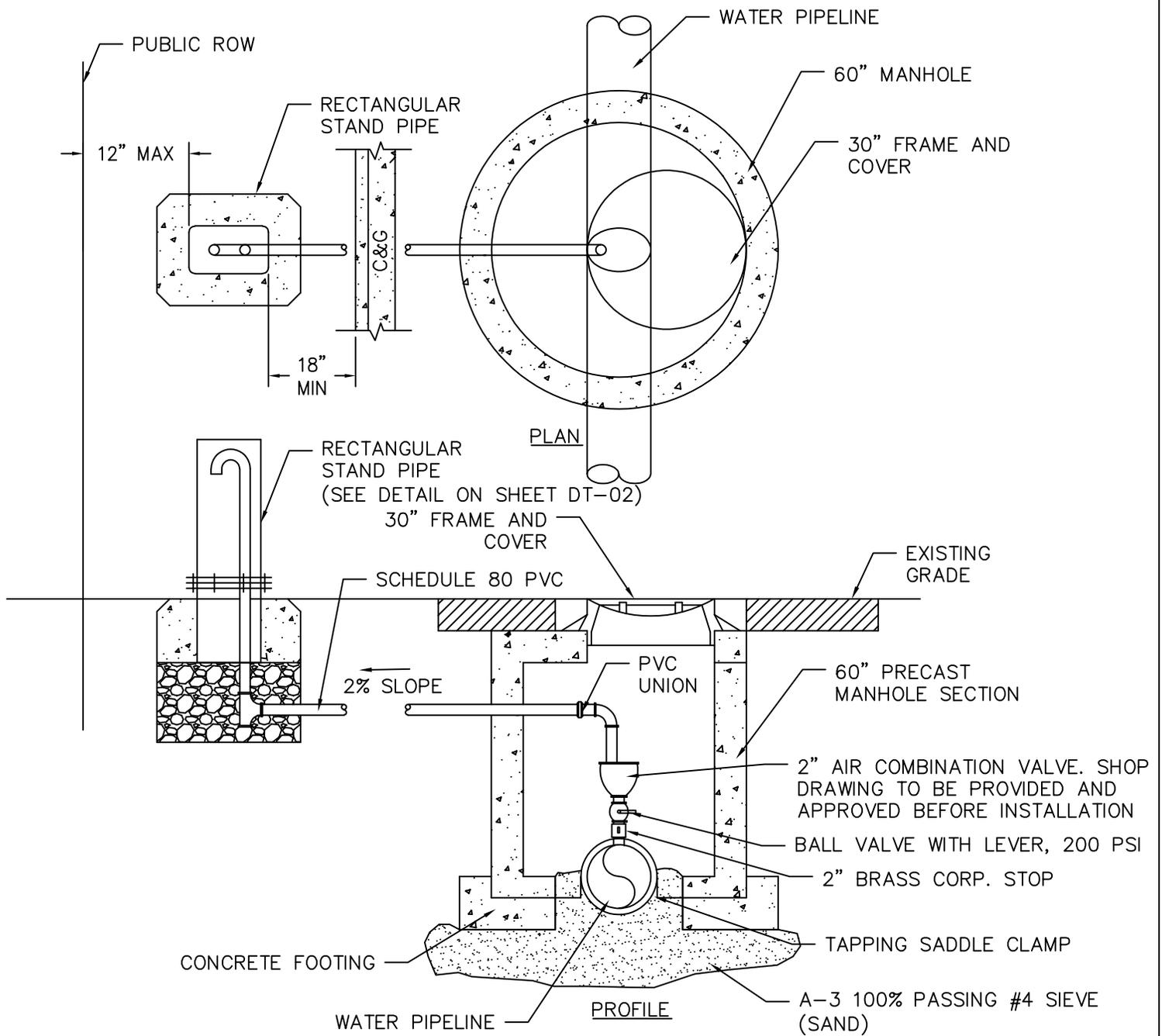
1. AIR VALVE STRUTURE: PLACE AIR VALVE STRUCTURE AT LOCATIONS SHOWN ON PLANS
