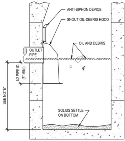
**NOTE:** SUMP DEPTH OF 36" MIN. FOR < 12" DIA. OUTLET. FOR OUTLETS > OR= 15", DEPTH = 2.5 TO 3 X'S DIAM.
