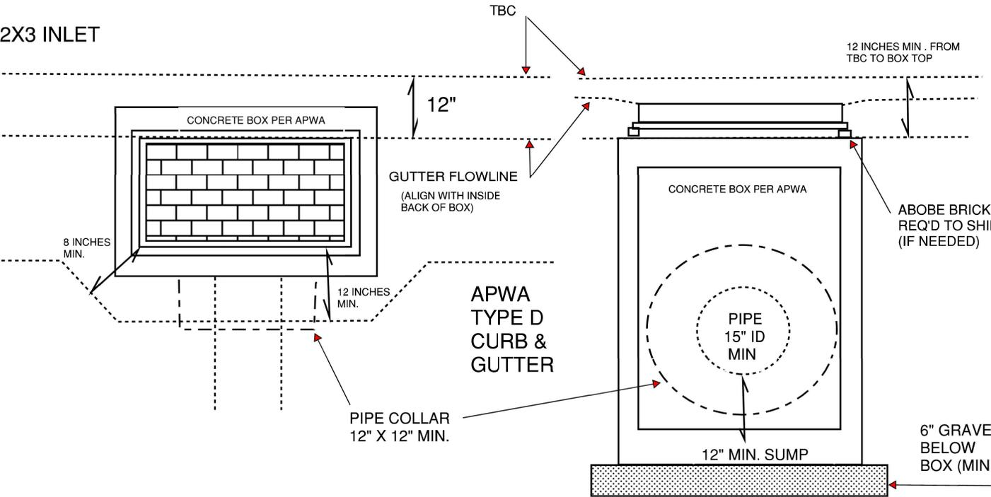
**BOX PLACEMENT FOR APWA TYPE A AND D CURB AND GUTTER**
